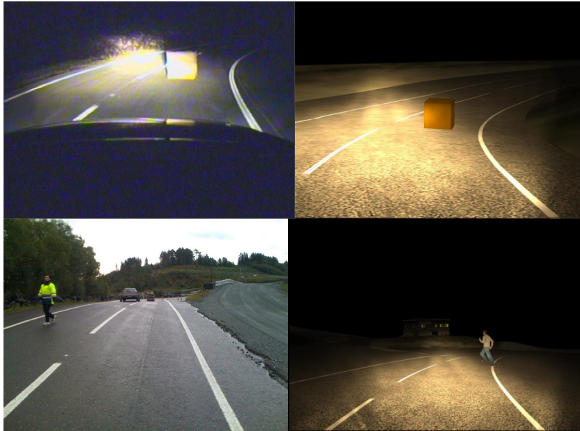
Figure 2: Upper panel: Example of the driver's visual impression of obstacle on the closed-circuit test track (left) and in the driving simulator (right). Lower panel: Visual Impression of pedestrian on test-track in daytime (left) and in driving simulator (right) during night-time. Note that the lower pictures are not taken in the same place or position.
