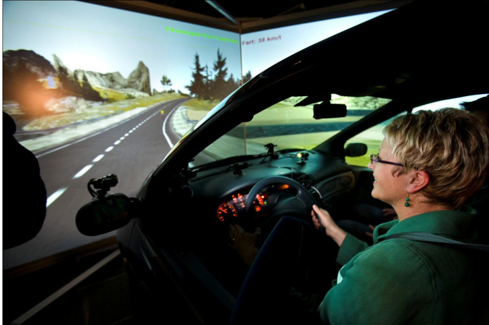
Figure 3. Setup of the driving simulator vehicle and surrounding frontal screens (photo by SINTEF)
