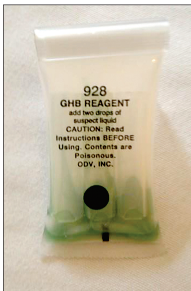
The NarcoPouch 928 GHB Reagent Test rendering a false positive after testing Dr. Bronner's Magic Soap.
